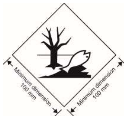
Environmentally hazardous substance mark
