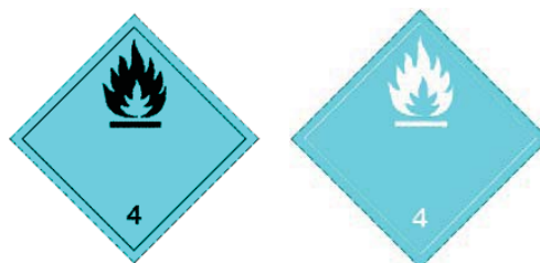
(No. 4.3) Symbol (flame): black or white; Background: blue; Figure "4" in bottom corner
